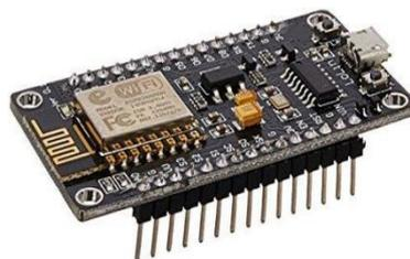
Gambar 2.3 NodeMCU
