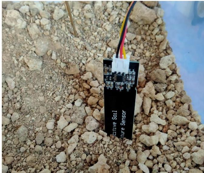
Gambar 4. 6 Sensor *soil moisture*
