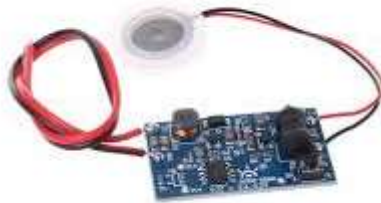
Gambar 2. 3 Ultrasonik mist maker (Sumber : Erisl Humidifier DIY Kit 5V Mist Maker Transducer Humidified Plate Accessories + PCB Module D16mm : Amazon.co.uk: Home & Kitchen)
