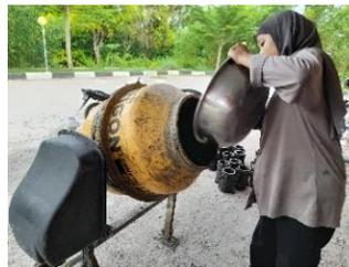
Gambar 3.12 Proses Mixing Campuran Benda Uji
