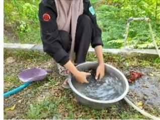
Gambar 3.4 Pencucian Agregat Kasar
