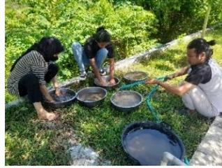
Gambar 3.6 Pencucian Agregat Halus
