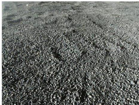
**Gambar 2.3** Aspal Buton Tipe B 50/30
