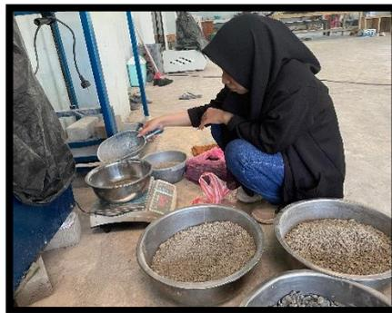
**Gambar 3.20** Menimbang masing-masing proporsi agregat
