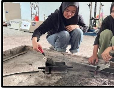
**Gambar 3.15** Pencetakan *paving block*
