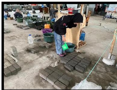
**Gambar 3.17** Perawatan *paving block*
