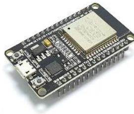
Gambar 2. 5 NodeMCU ESP32
