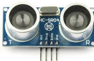
Gambar 2. 8 Sensor Ultrasonik
