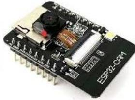
Gambar 2. 5 *ESP32 Cam*
