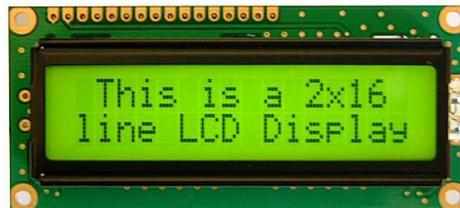
Gambar 2. 9 *LCD (Light Crystal Display)*
