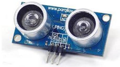
Gambar 2. 2 Sensor ultrasonik
