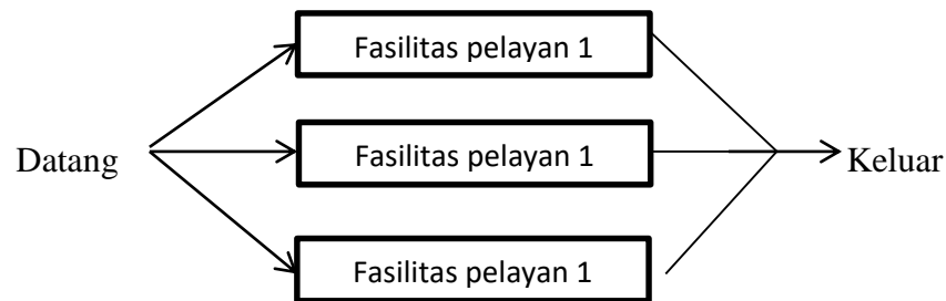
Gambar 2.3 model Multi channel – single phase Nurfitriani et al. , 2017
