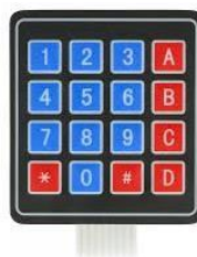
Gambar 2. 6 Matrix Keypad 4x4
