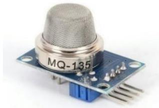
**Gambar 2. 4** Sensor CO<sub>2</sub>
