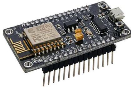
**Gambar 2.2** NodeMCU ESP8266
