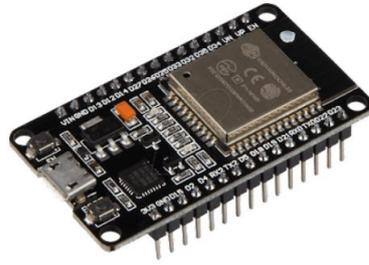
*Gambar 2. 5 NodeMCU ESP32*
