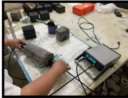
**Gambar 2.2** Uji *Ultrasonic Pulse Velocity Test* (Sumber : Dokumentasi Pengujian di Laboratorium)
