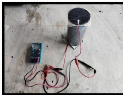
Gambar 2.4 Uji *Electrical Resistivity* Silinder
