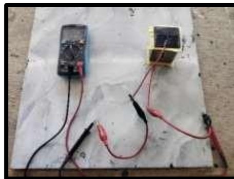
Gambar 2.5 Uji Electrical Resistivity Kubus 5 cm x 5 cm x 5 cm Beton Umur 56 hari
